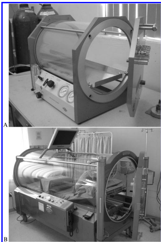
Figure 1: (A) A typical bench-top small-animal hyperbaric oxygen chamber; (B) a human hyperbaric oxygen chamber. The patient lies supine during therapy, and is able to watch the television monitor on top of the unit for entertainment
